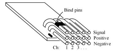
Receiver should be considered 'experimental' and used at own risk. Protect from vibration e.g. with velcro or foam mounting.
